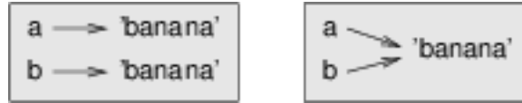
Figure 11.1: Variables referring to different objects, and variables that refer to the same object.
